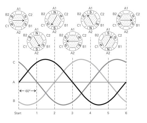
The speed of the rotating magnetic field is referred to as synchronous speed (Ns). Synchronous speed is equal to 120 times the frequency (F), divided by the number of poles (P).
