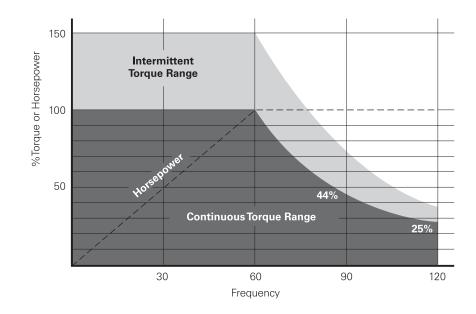
The sample motor described above is capable of operating at 100% rated torque continuously at low frequencies. Many motors are <u>not</u> capable of operating continuously at 100% continuous torque at low frequencies. Each motor must be evaluated before selecting it for use on an AC drive.
