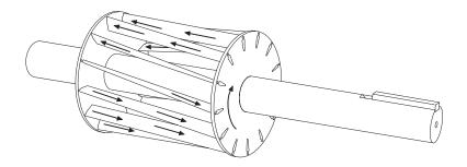
There must be a relative difference in speed between the rotor and the rotating magnetic field. The difference in speed of the rotating magnetic field, expressed in RPM, and the rotor, expressed in RPM, is known as slip.
