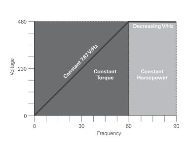
Horsepower remains constant as speed (N) increases and torque (T) decreases in proportion. The following formula applies to speed in revolutions per minute (RPM).
