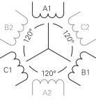
2-Pole Stator Winding
