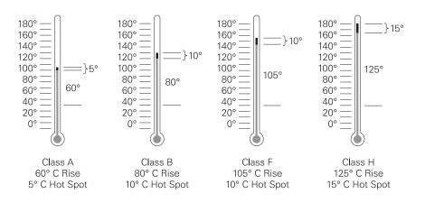
The operating temperature of a motor is important to efficient operation and long life. Operating a motor above the limits of the insulation class reduces the motor's life expectancy. A 10° C increase in the operating temperature can decrease the life expectancy of a motor as much as 50%.
